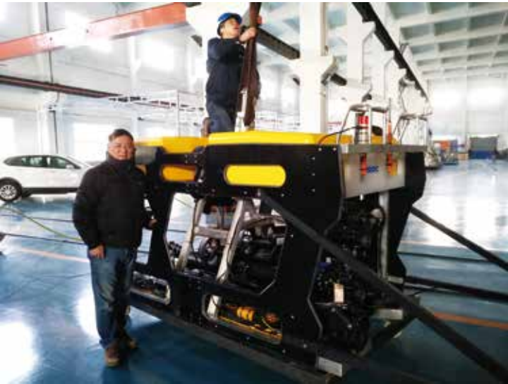
方励主持研制的DeepOcean X8深海作业级电动水下遥控机器人。 DeepOcean X8 Electrical Work Class ROV designed by Fang Li.
