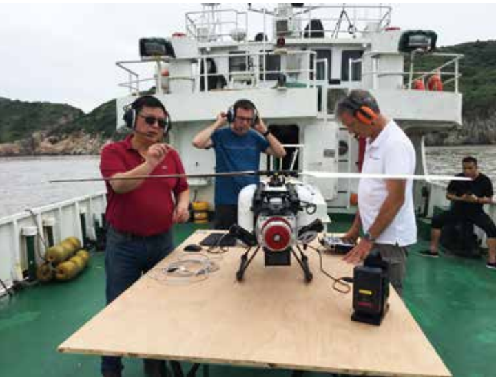
方励与他控股的比利时Flying-Cam无人直升机公司技术人员在舟山群岛进行超轻型无人直升机载三维激光扫描岛礁测绘演示。 Together with his technical team from Flying-Cam AS in Belgium, Fang Li is demonstrating island survey by 3D laser scanner loaded on their ultra-light unmanned helicopter in Zhoushan.
