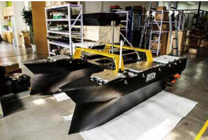
方励主持研制的H-3000型无人自主海洋测绘艇。 H-3000 Hydrographic Survey ASV designed by Fang Li.
