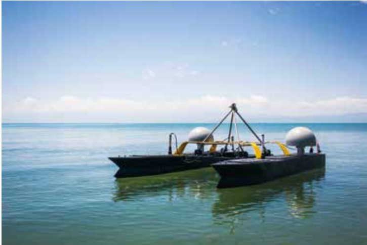
自主研制的无人自主多波束海洋测绘系统在青海湖进行水下三维地形测绘。 Hydrographic Survey in Qinghai Lake with ASV based multibeam echo sounder system.
